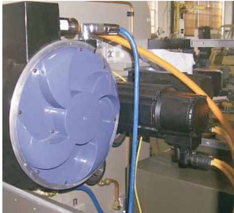
Cartridge DDR motors from Kollmorgen mount directly onto a converting machine, using the machine's existing bearings to support its rotor.
