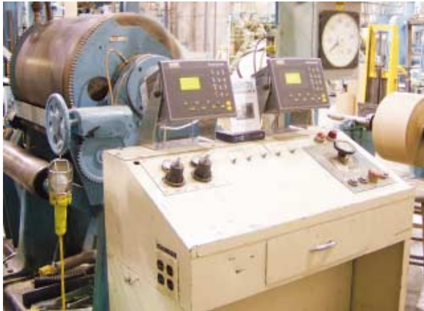
At Georgia Tech's Institute of Paper Science & Technology, tension control had been a problem on a corrugated line. Here, Hardy Instruments HI 3600 tension controllers, installed at the operator's console, help provide precision control at all times.
