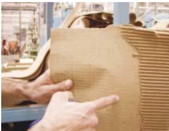
An example of inferior corrugated bonding due to poor tension control. Georgia Tech's IPST conquered this problem with help from Hardy Instruments.
